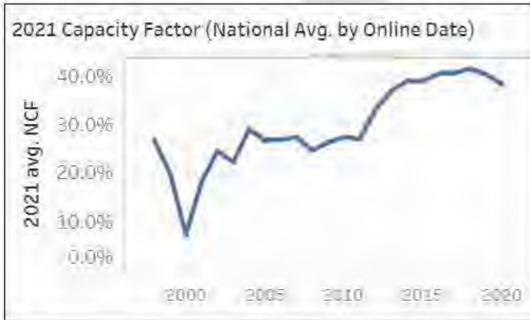
Figure D-12. This figure shows capacity factors for U.S. onshore wind turbines by the year they entered service. In no year do these turbines reach EPA’s assumed 42.2 percent capacity factor on an annual basis.
