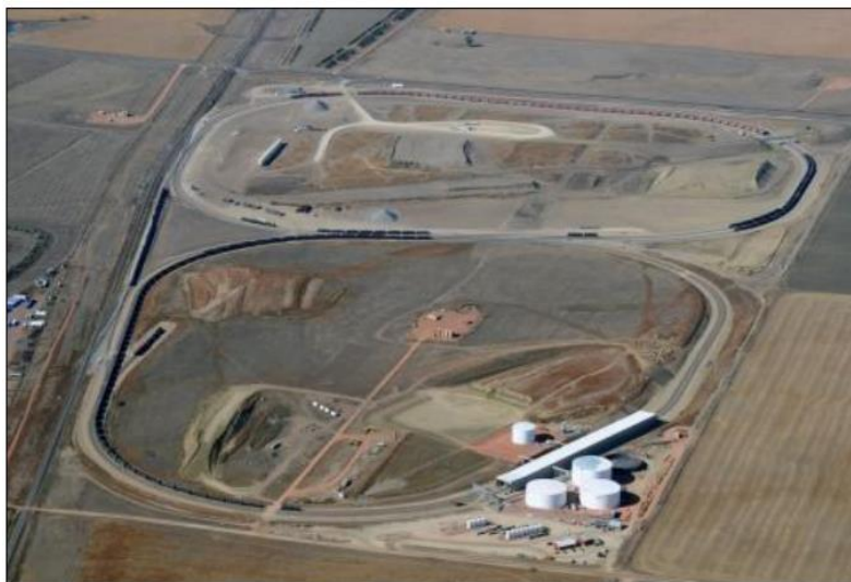
Figure 3.15-2. Example Crude Oil Rail Loading Terminal
