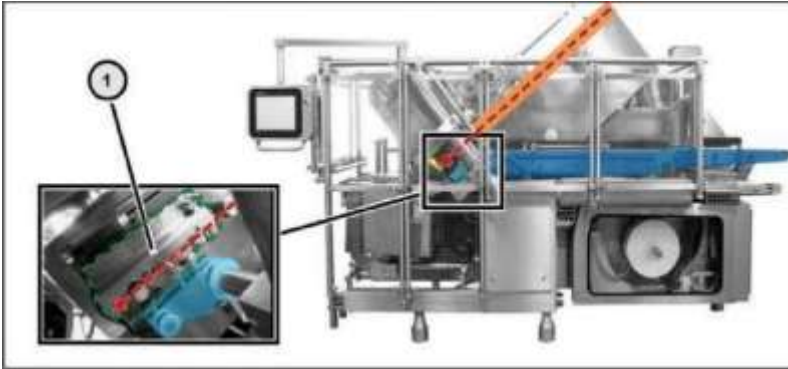
Fig. 10 Position of the product bed conveyor
