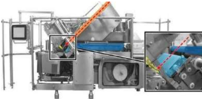
Fig_ 227 Position of the product bed conveyor
